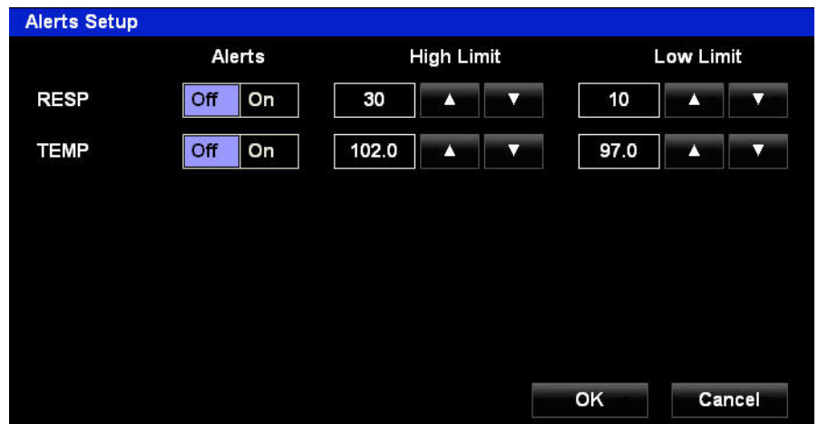
Figure 2-5 Alerts Setup window, RESP and TEMP settings
