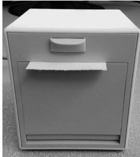
Figure 4-4 Recorder with paper correctly installed
