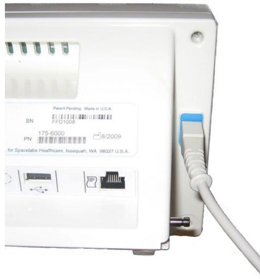
Figure 4-2 SpO<sub>2</sub> Adapter Cable Connected to Ultraview DM3 Monitor
