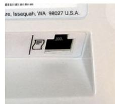
Figure 9-1 Connector for Strip Chart Recorder
