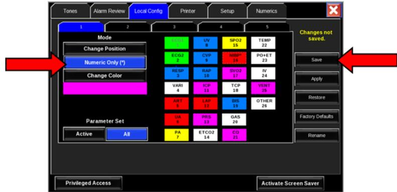
*Note: A Numeric Only parameter is noted with an asterisk on the parameter label.*
