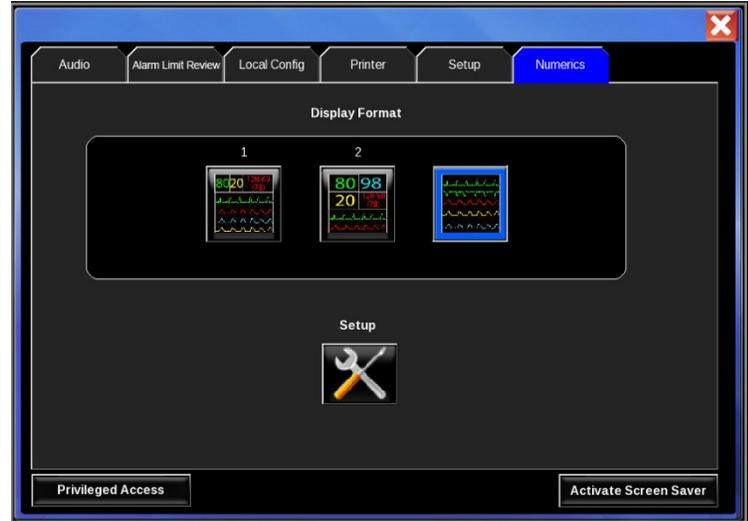
To configure the Large Numerics display with the parameters you want to view
