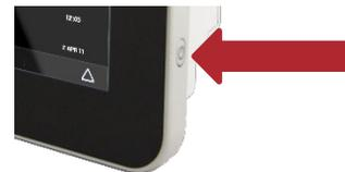
2. To power the monitor OFF, press and hold the ON/OFF button until the screen turns off. A pop-up will present a red bar that will advance until the monitor has turned OFF.
