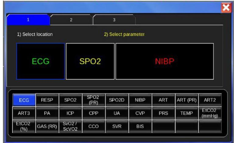
*Note: The tabs at the top allow you to view and configure the different displays. However, the view selected in the NUMERICS tab is the view that will be presented on the monitor.*
