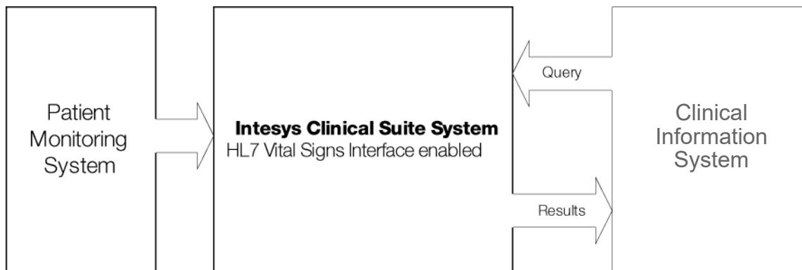
The Vital Signs Interface transfers vital signs data from Spacelabs Healthcare monitors and attached peripheral devices to a hospital clinical information system (CIS). The interface provides solicited and unsolicited Health Level Seven (HL7) result messages to the destination system at a rate that is configurable by clinical unit. The Vital Signs Interface is an integrated component of the Intesys® Clinical Suite (ICS).
