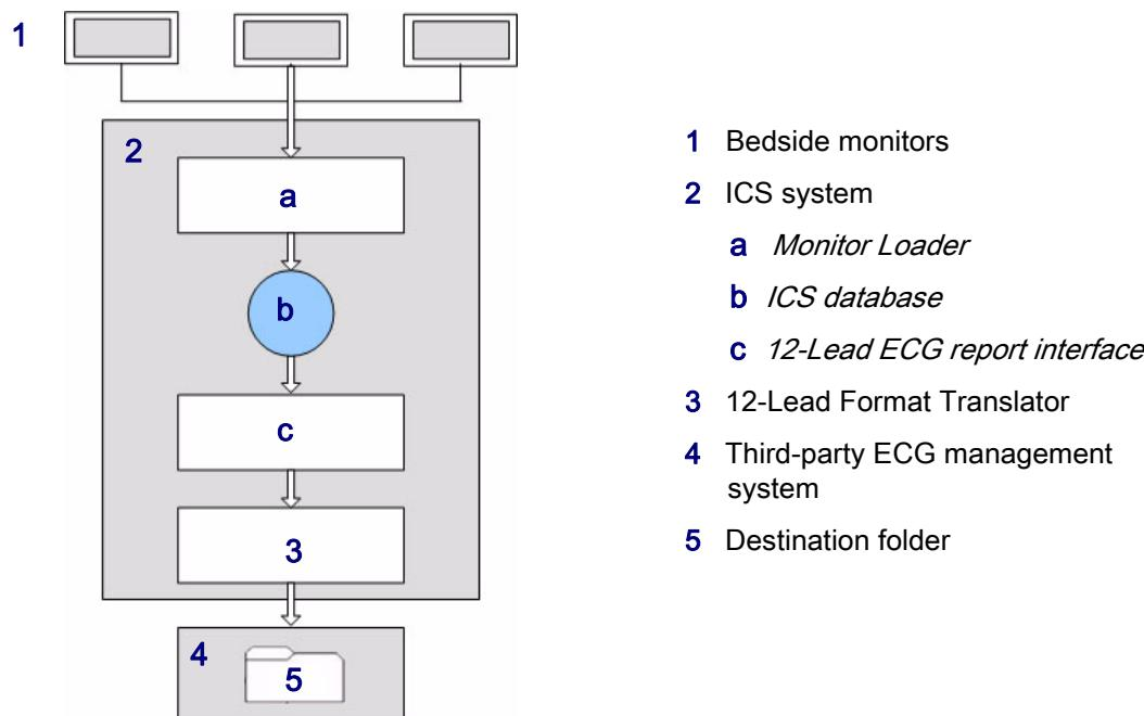
The 12-Lead Electrocardiogram (ECG) Interface is a product in the Intesys® Clinical Suite (ICS). This interface enables Spacelabs Healthcare patient monitors, with 12-Lead capability, to send 12-Lead reports to an ECG management system.
