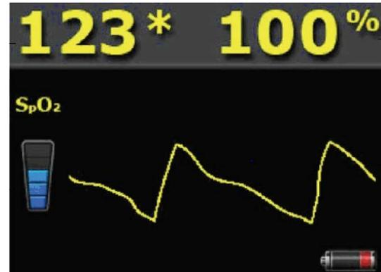
*NOTE: SpO<sub>2</sub> automatically shows on the Xhibit™ Central Station when the SpO<sub>2</sub> cable is connected to the transmitter. To show SpO<sub>2</sub> on Ultraview SL™ monitors, select **ECG > CHANNEL FORMAT > SpO<sub>2</sub> ON/OFF**.*
